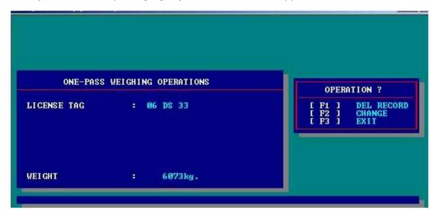
Here pressing **[F1]** key will delete this definition. If you do this LM 6 will ask you to confirm deletion. You can confirm deletion by pressing **1** or decline it by pressing **2**.
