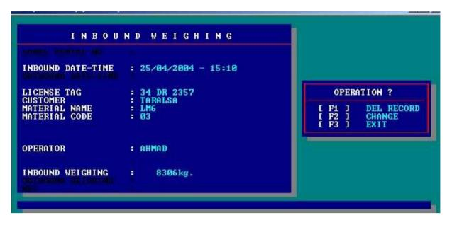
Here you can delete this record by pressing [F1] key or make changes on this record by pressing [F2].
