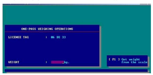
After typing the license tag number and confirming it with [ENTER] key terminal will ask you to enter the tare of the truck. You can either enter it by typing directly or get the tare weight from the scale by pressing **[F1]** key. After confirming the tare weight with [ENTER] key you will automatically get back to the operations of the one-pass weighing operations submenu.
