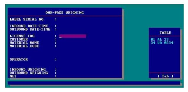
Select the desired truck from the predefined table at the right side of the screen and press enter to perform weighing.
