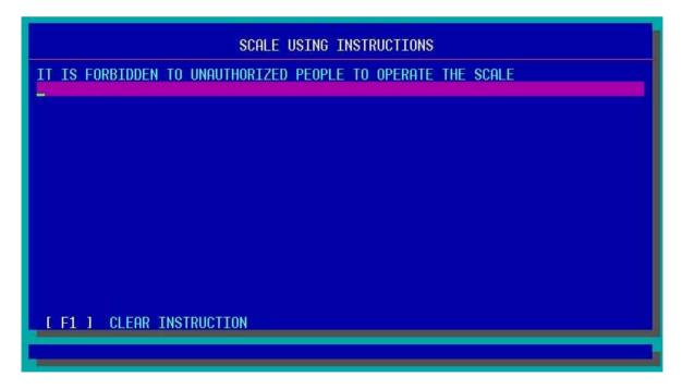
Here you can write instructions to the operator that will be seen for 15 seconds at the beginning as you turn the terminal on.
