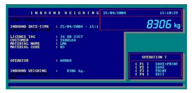
As you enter the inbound weighing menu LM 6 will ask you the LICENSE TAG of the truck. After entering the truck you will enter the entries and operator info and press ENTER to perform weighing. A new window appears at the right bottom of the screen.
