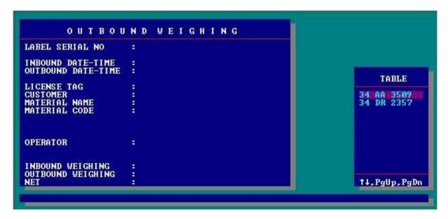
When you enter the outbound weighing menu the license tags of the trucks of which inbound weighings had been made will be given in the table on the right side in alphabetical order. Press [TAB] key to get into the table and select the truck that you will make the outbound weighing by using arrow keys and accept by pressing the enter key. If you begin to type the tag, the table gets in to a new order that only includes the tag numbers that you have already typed.
