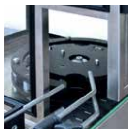
Rotational feeder of cylindrical products
